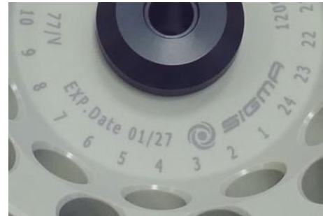
Fig. 4: Different service life – engraving on the bucket/rotor
